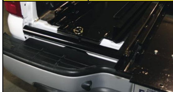
Ramps are pinned and stored in the pickup bed when not in use.
