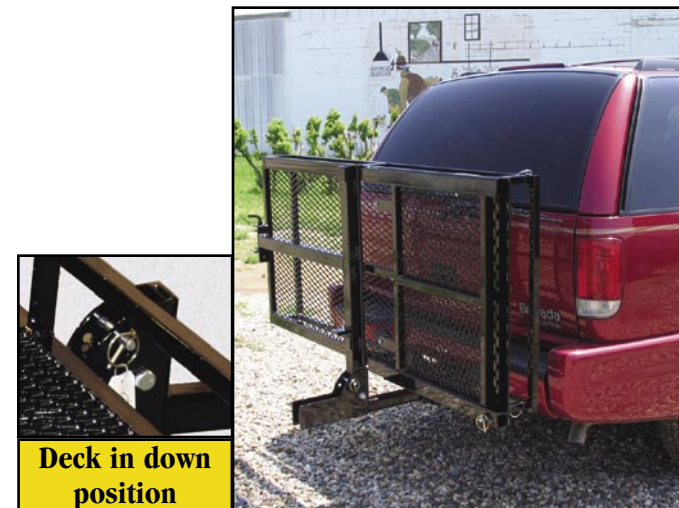
Pin is replaced after putting the carrier in the folded position
