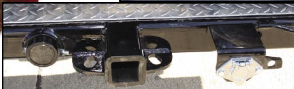
Receiver is built in allowing to tow from the deck and electrical connection
